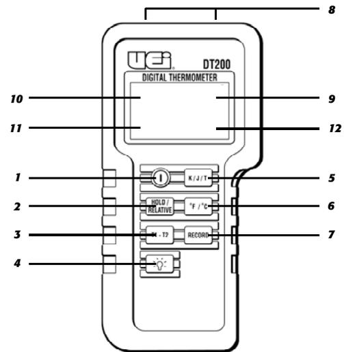
1. **Power Switch:** Powers instrument on and off.
